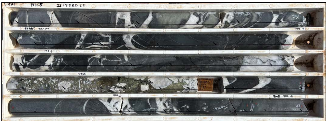
Figure 5: 22PTMRD011 from 750.07 – 754.61 m showing the typical quartz-carbonate breccia that dominates the hole from 705 – 826 m. Drilling had intersected a section of massive sulphide within brecciated quartz and carbonate matrix from 752.7 – 753.5 m. Sulphides here comprise of chalcopyrite-pyrite-pyrrhotite
