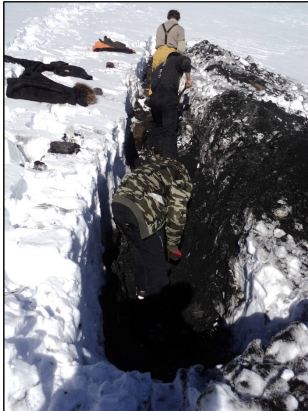
Figure 5-11: Clearing away weathered coal
