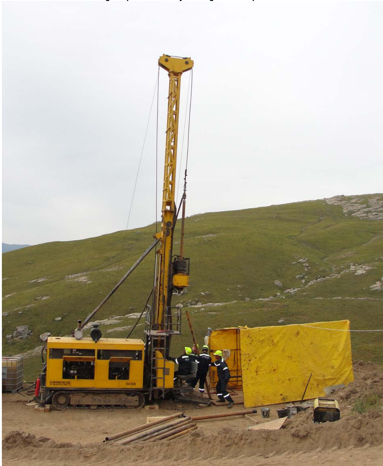
Diamond core drill rig in operation at Tuyuk-Kargasha Prospect – Drillhole DD12TK001
