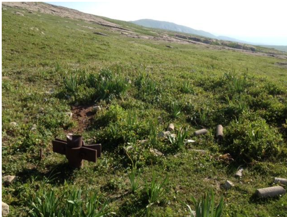
Soviet Era Drillhole Collar and Diamond Core
