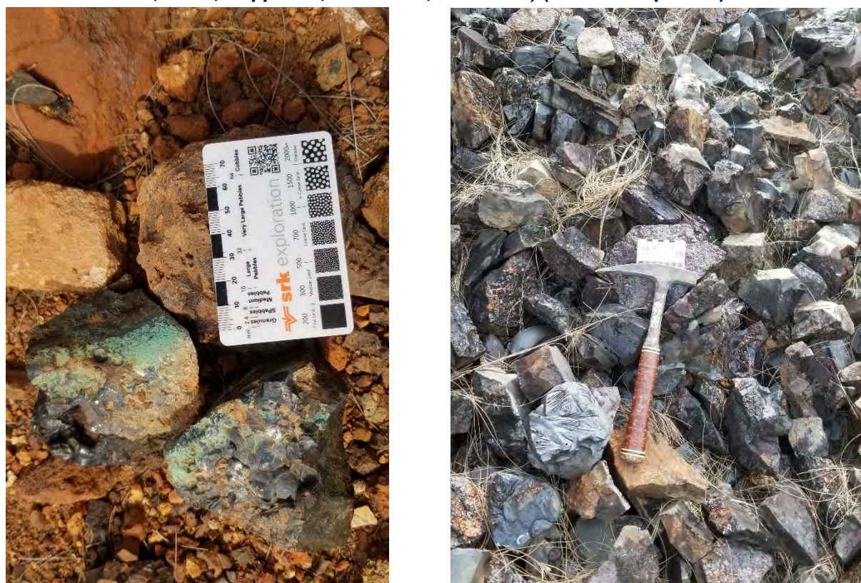
Figure 3-24 Using pXRF to verify the grade range of slag fragments from the dump (left to right; 954ppm As, 6,180ppm Cu, 3.013% Zn; 925ppm As, 6,210ppm Cu, 3.035% Zn; and 1,832ppm As, 1.938% Cu, 2.107% Zn) ( SRK ES Sept 2019)
