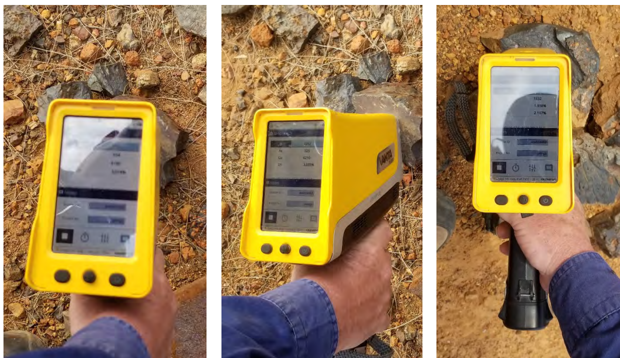
Figure 3-24 Using pXRF to verify the grade range of slag fragments from the dump (left to right; 954ppm As, 6,180ppm Cu, 3.013% Zn; 925ppm As, 6,210ppm Cu, 3.035% Zn; and 1,832ppm As, 1.938% Cu, 2.107% Zn) ( SRK ES Sept 2019)
