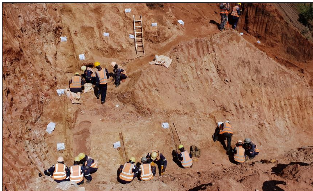
Figure 9-7 Channel sampling on a REE vein at Gasagwe Mine
