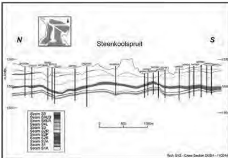
Figure 5.9: Cross-section through Steenkoolspruit pit
