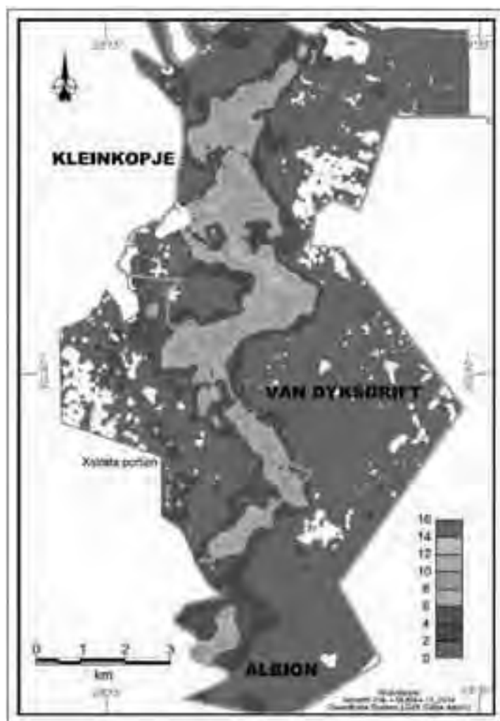
Figure 5.5: Distribution and thickness of prominent sandstone channel at Wolvekrans – legend shows interburden thickness between No.2 Seam and No.2A Seam in metres
