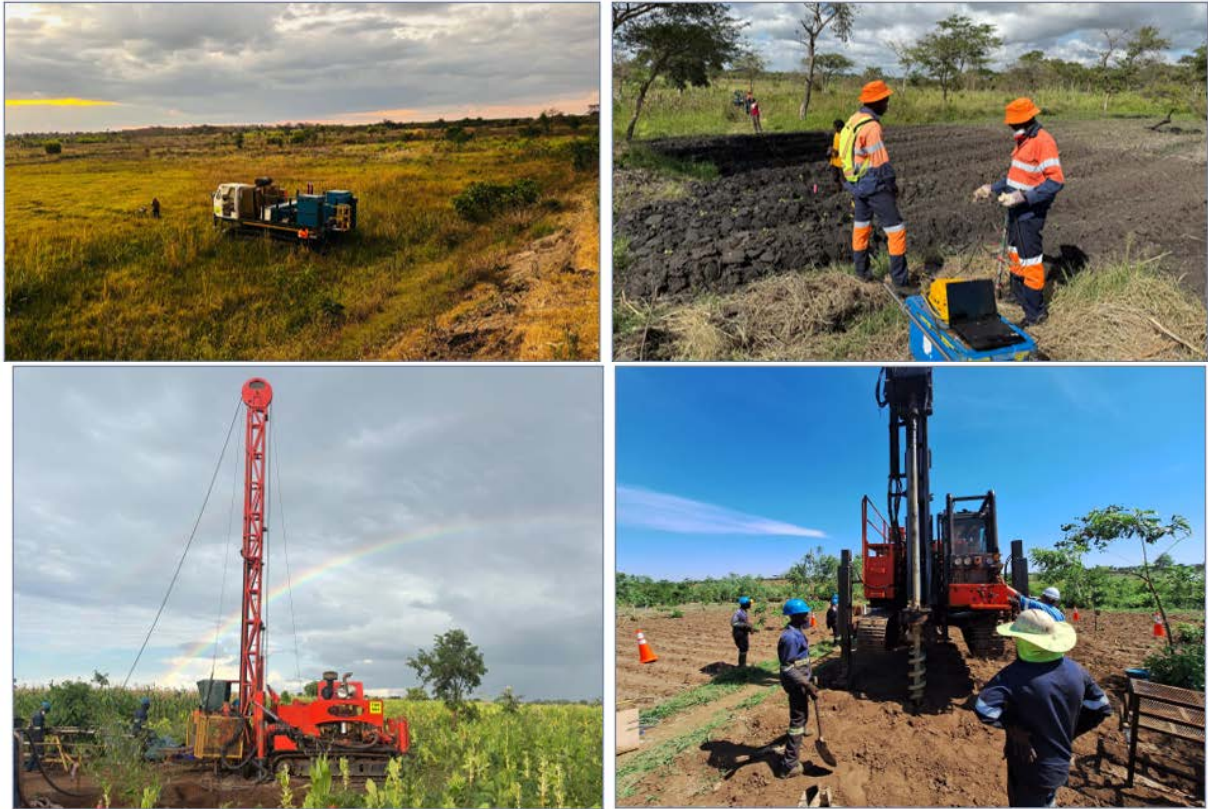
Figures 3-6 Clockwise from Top Left: Geotechnical diamond drilling, auger drilling, seismic geophysics testing using multi-channel analysis of surface waves (MASW), Cone Penetration Test with pore pressure measurements (CPT) rig.
