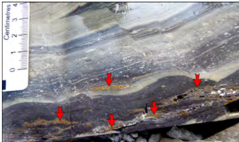
Figure 7-15 High grade intersection at Ivanhoe Mines Ltd Kamao Project showing lenses of chalcopyrite-bornite (e.g., as indicated by arrowheads) within the weakly deformed host siltstones and reworked glacial sedimentary rocks that constitute the main host in the Grand Conlomérat of the basal Nguba Group
