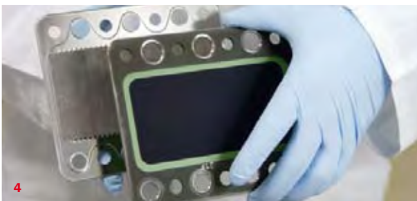
4 Fuel cell In a fuel cell drive system, the fuel cell employs a chemical reaction to generate the electric power for an electromotor which drives the vehicle or equipment.
