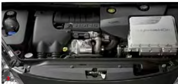
3 Hybrid drive The internal combustion engine and the electromotor are combined in the hybrid drive. Generating and converting energy and the subsequent release of that energy occur at different times; the energy is buffer-stored in a battery.
