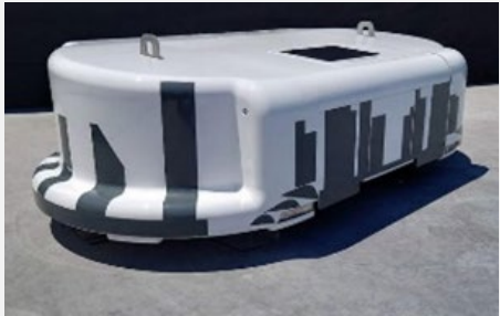
Floor Finishing Robot
