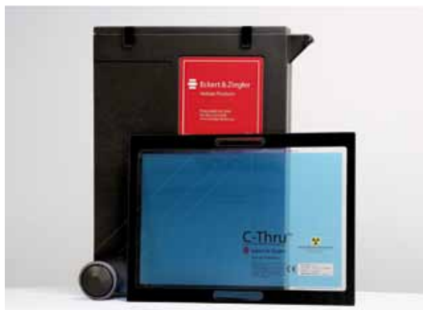
Flood source for the calibration of diagnostic cameras used in nuclear medicine
