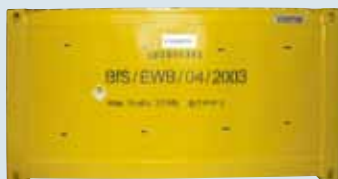
Konrad container suitable for final disposal
