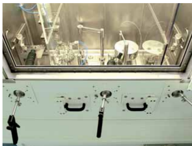
Dispensing unit for Yttriga, pharmaceutical grade Y-90
