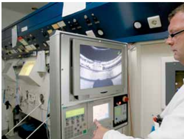
Laser welding of Sr-90 radiation sources
