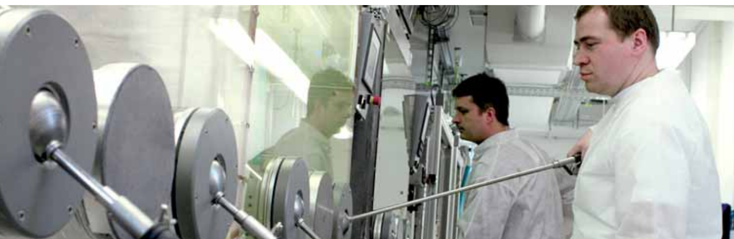
Production line for producing low level radioactive prostate implants
