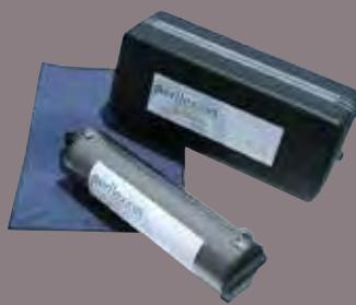
*Perfexion™: a unique flexible radiation source used in the calibration of nuclear medicine imaging equipment*
