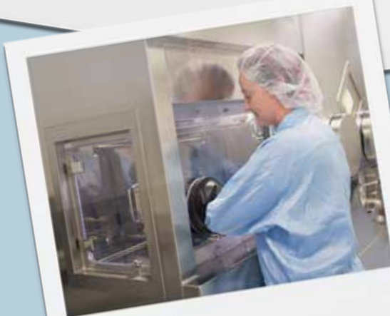
Production of GalliaPharm 68Ga radio nuclide generator in the clean room
