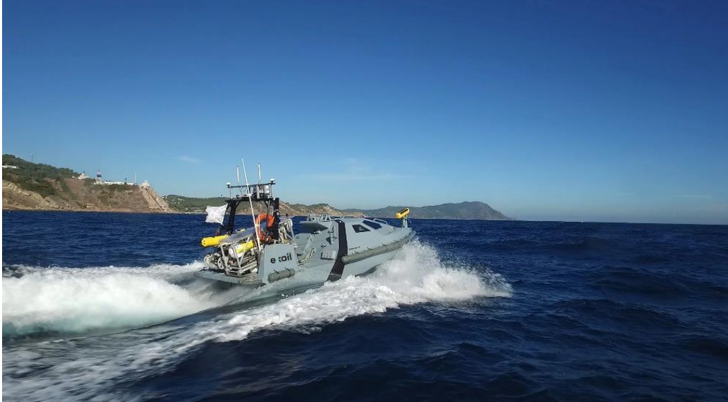
Surface drone USV Inspector 90 and its Launch & Recovery system
