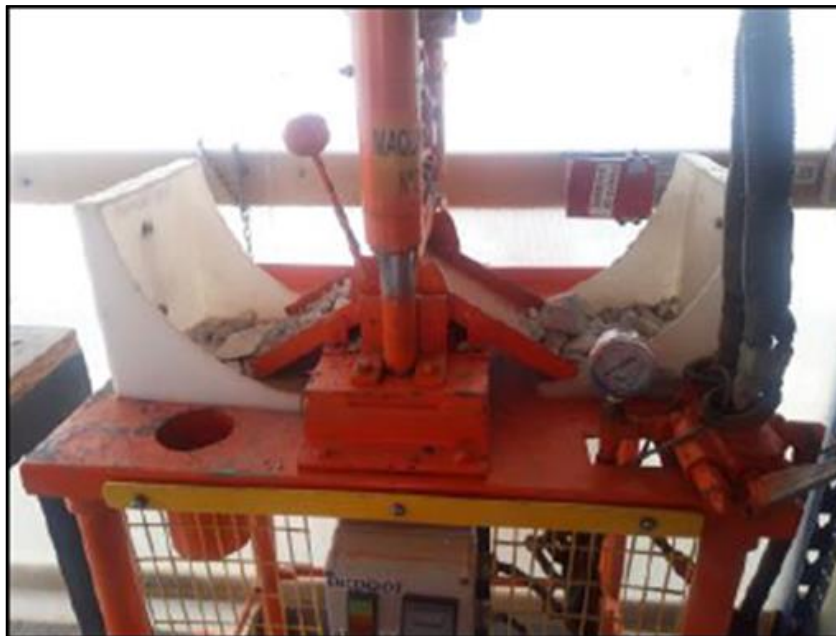
Figure 8-5: Hydraulic Guillotine for Core Cutting
