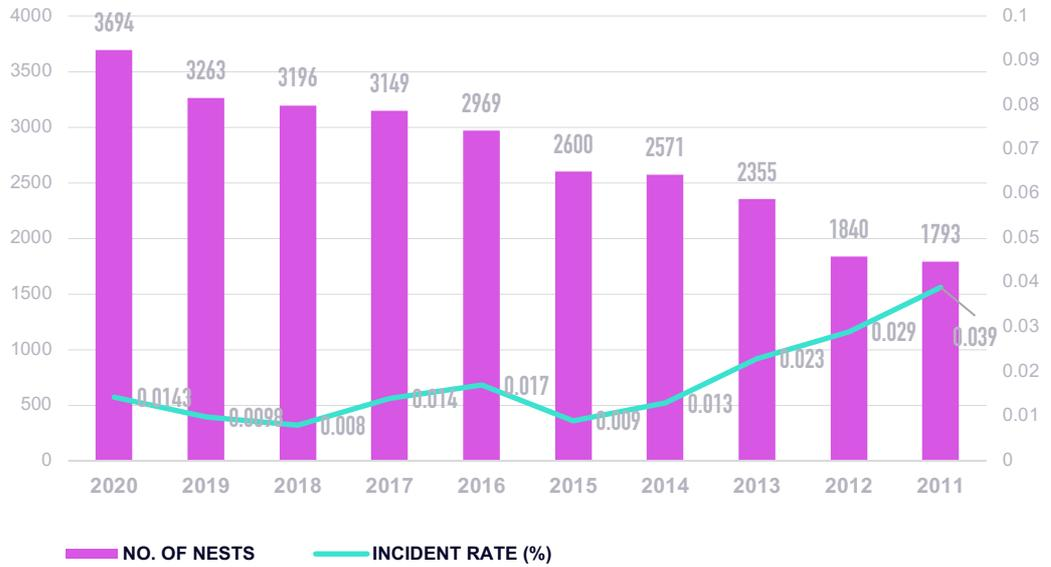
The fitting of fans and platforms stops nesting in places with greater likelihood of incidents, i.e., despite the constant increase in the population of storks causing a relevant increase in the number of nests, the number of incidents has remained stable and low.
