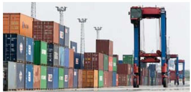
Diesel-electric van carriers on Burchardkai.
