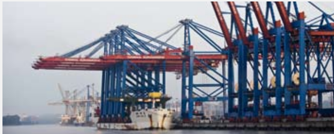
New "twin-forty" container gantry cranes for Burchardkai.
