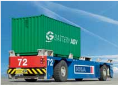
Automated guided vehicles (AGVs) emit 30 percent less CO 2 thanks to hybrid diesel-electric engines. The next generation of vehicles could be battery powered if the trial proves successful.
