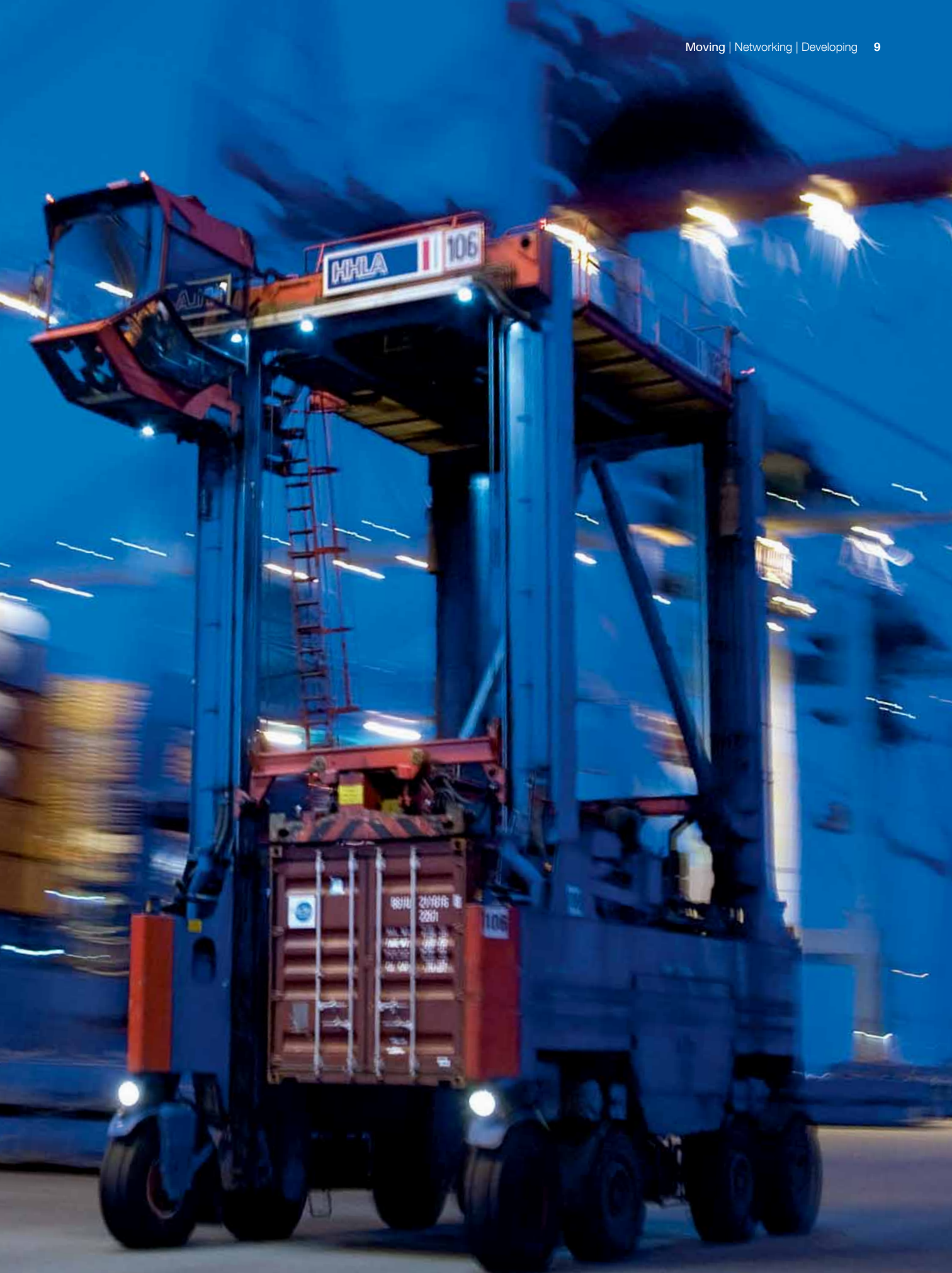
Straddle carriers transporting a container at the HHLA Container Terminal Burchardkai.
