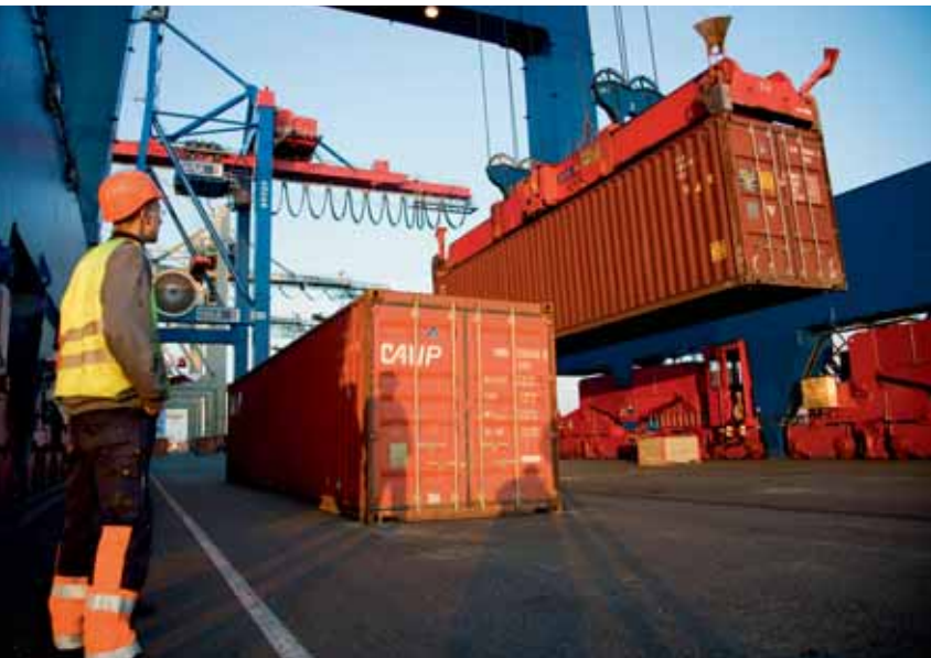
Containers are deposited on the quayside before straddle carriers take them to the yard.
