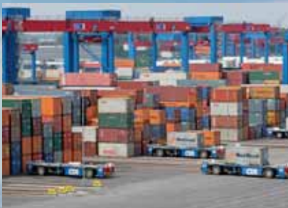
Automated storage blocks, operated by rail-mounted gantry cranes, opens up new possibilities for the efficient use of space. Only half the conventional amount of yard space is needed per container.
