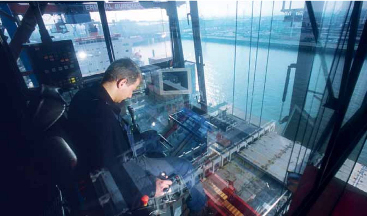
The operator of a container gantry crane unloading the containers.
