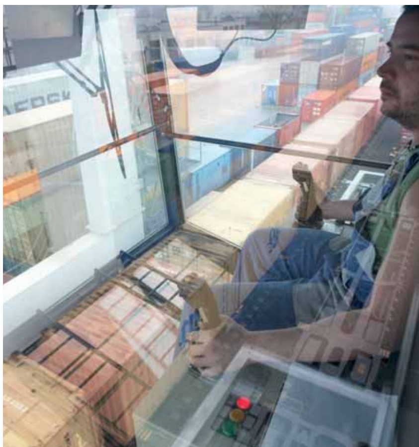
A crane operator in the cab of a rail-mounted gantry crane at the Metrans terminal in Prague.
