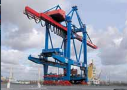
Semi-automatic double-trolley container gantry cranes have generators which recover electricity when the container is lowered, saving 20 to 25 percent of their energy needs.
