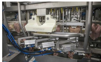
AMF-i breast cap filleting system
