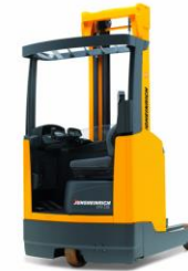
Elektro- Schubmast- stapler
