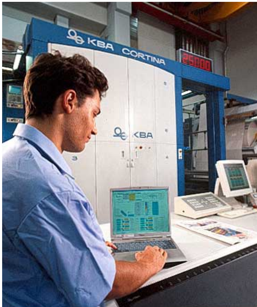
The world's first double-width waterless newspaper press went into operation at reiff zeitungsdruk, Offenburg, in autumn 2002
