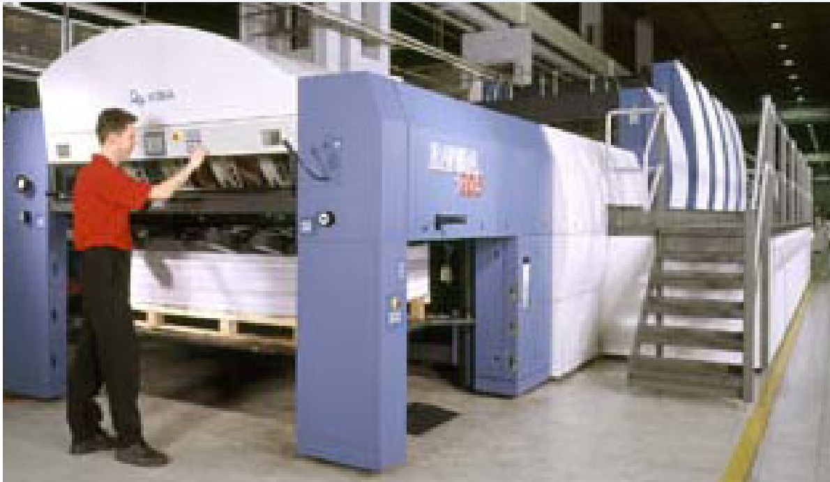
The superlarge Rapida 205 launched at the end of the year is the biggest sheetfed press worldwide and offers poster, display and packaging printers a whole new perspective
