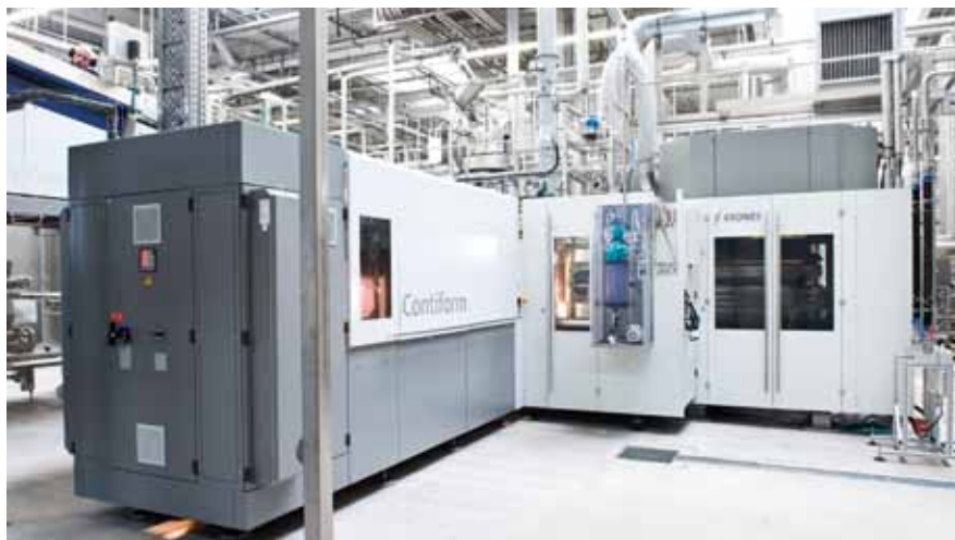
The Contiform stretch blow-moulder is now even faster and more efficient.
