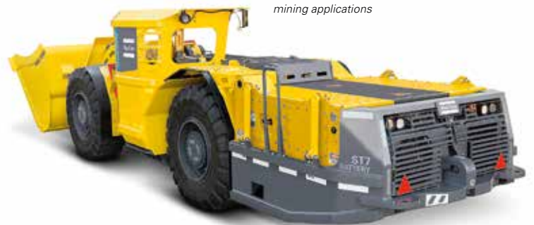
Battery-driven underground loader for mining applications
