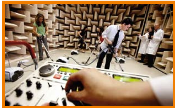
On the basis of these insights, Electrolux decided to develop a silent vacuum cleaner. New technology focused on air-flow enhances performance and reduces the noise level. The unit also features extra insulation for the motor, as well as shock-absorbers. The vacuum cleaner is so silent, one can easily listen to music while vacuuming.
