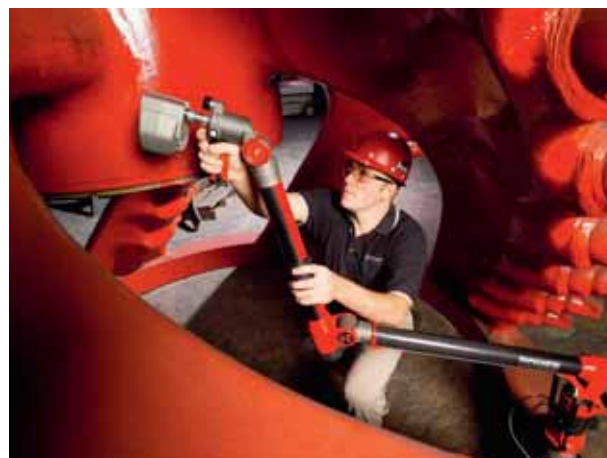
Portable measuring arms offer total flexibility and mobility. This Romer measuring machine is brought to the work piece – not the other way round.
