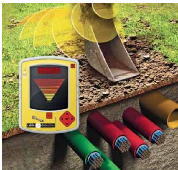
In February 2008 the Hexagon subsidiary Cable Detection launched EZiDIG, the world's first excavator mounted cable avoidance tool to add a crucial level of safety to the excavation process. The product won several innovation awards during the year.
