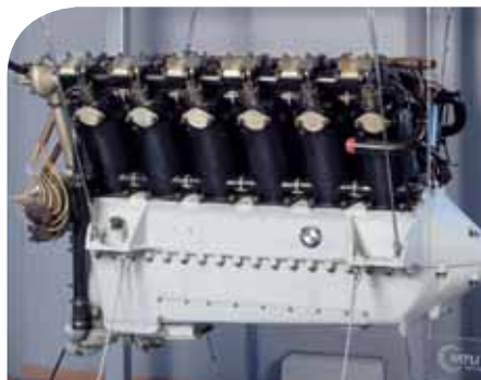
Standard engine of many historic German aircraft: the BMW VI.
