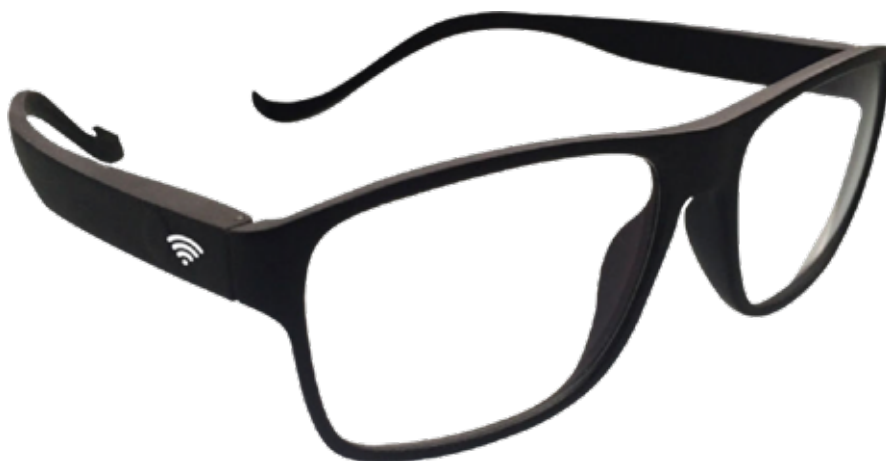
Glasses with sensors for medical use. If the wearer falls, a signal is sent to a remote monitoring platform that alerts family members or medical care.
