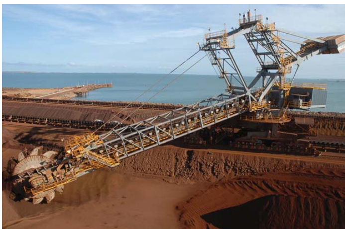
Material processing facilities represent some of the investment-related project solutions offered by Sandvik Mining and Construction. The picture shows a Sandvik Reclaimer PR200 working in Port of Dampier in Parker Point, Australia.
