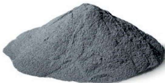
METALLIC POWDER USED FOR MANUFACTURING HIP COMPONENTS
