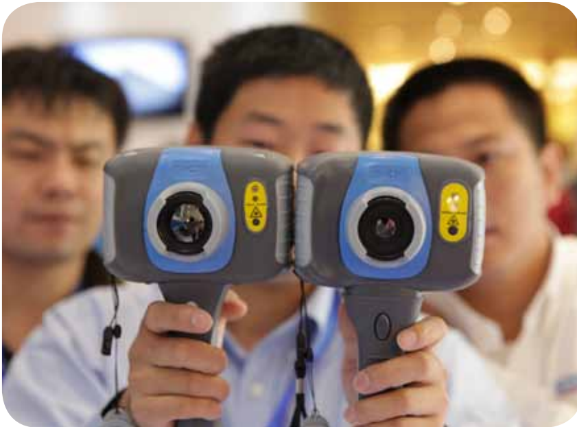
Participants at the Distributor Development Conference in Beijing, China, testing SKF Thermal Camera TKTI 20, which has an infrared detector. Thermal imaging is used by many industries as a predictive maintenance technique.
