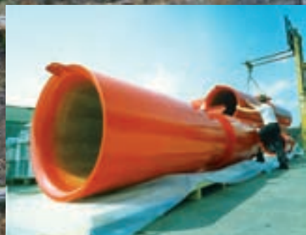
Systemair's tunnel fans are manufactured at the production plants in Germany and Malaysia. During 2009, 328 tunnel fans were delivered for the A32 motorway in Italy.
