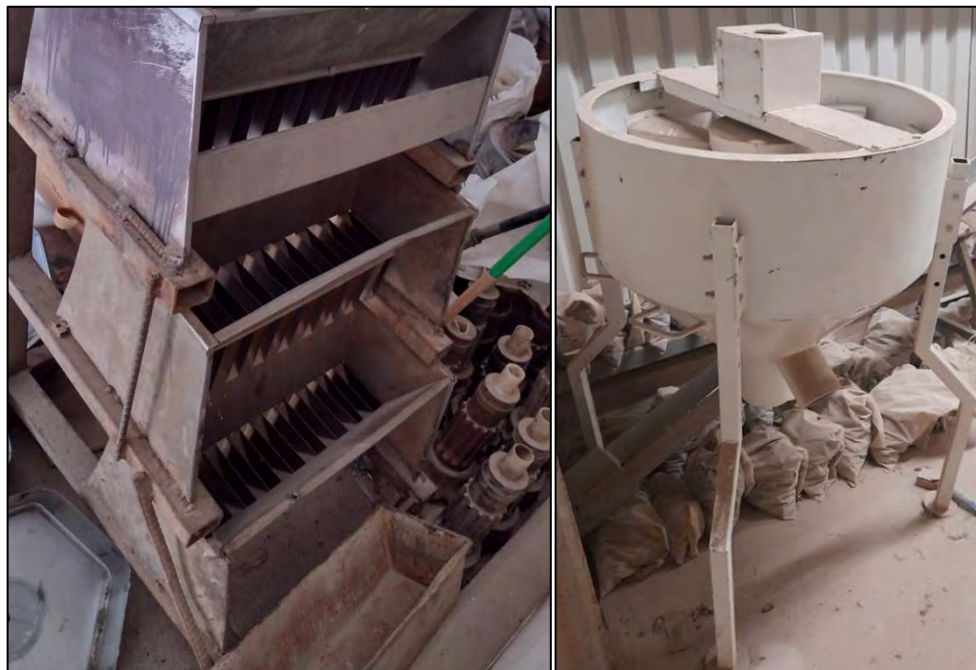
Figure 8.1: Jones Splitter – RC Sample Splitter, Left, Mechanical Splitter, Right
