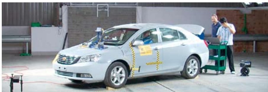
A vehicle under preparation for full-scale crash test in Autoliv's new technical center in Shanghai, China.
