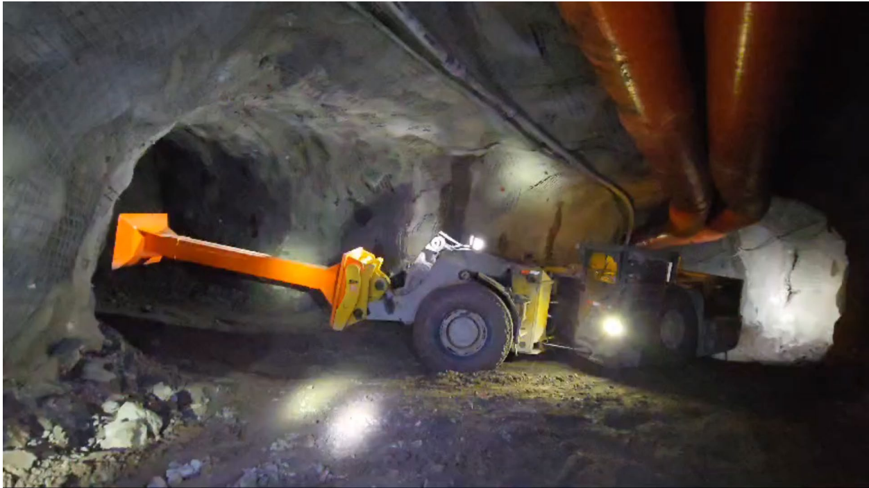
Figure 13-7: Scoop Fitted With A Rammer Plate
