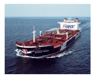
The *Stena Paris* is one of ten P-MAX tankers in Concordia Maritime's fleet. The vessels have a double hull, two engine rooms with full water and fire integrity and two separate propulsion systems. Manoeuvrability and an integrated bridge layout are also very important when it comes to facilitating safe navigation in narrow channels.
