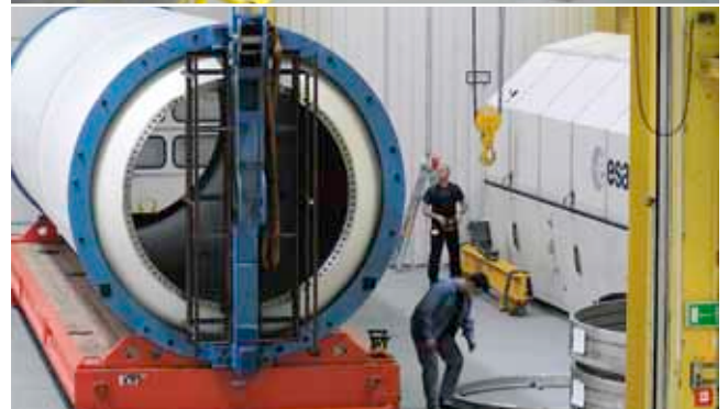
Production of Ariane 5 booster cases at MT Aerospace in Augsburg
