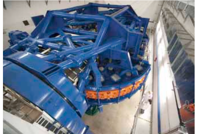
The Heidelberg Ion Radiation Therapy Center HIT. MT Aerospace provided the world's first rotating gantry.
