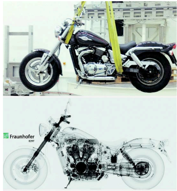
First light tested on a motor cycle using the new X-ray technology
