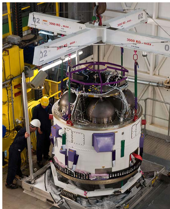
Integration of the current VEGA VV02 AVUM upper stage in Kourou
