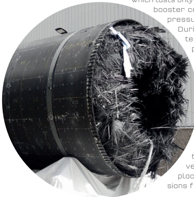
Component after the successful bursting test at MPA in Stuttgart
