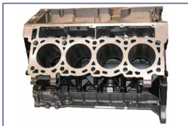
The Navistar 6.4 Litre V8 cylinder block began series production at the Cifunsa foundry in Mexico during 2009 (Courtesy, Navistar)
