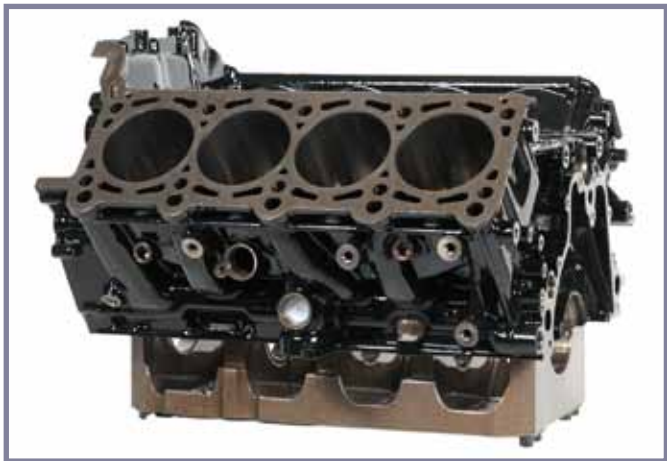
The Audi 4.2 Litre V8 cylinder block began series production at the Halberg foundry in Germany during 2005. The 4.2 Litre V8 is an upgrade of the 3.3 Litre V8, the first-ever series production CGI cylinder block, launched in 1999 (Courtesy, Audi)
