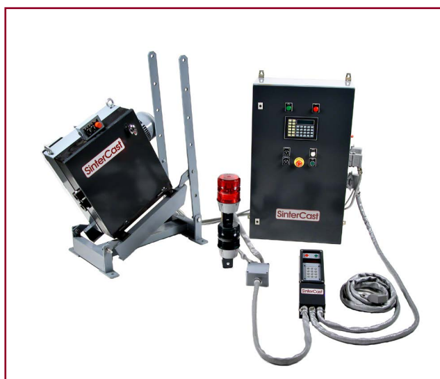
Automatic wirefeeding for base treatment and correction
