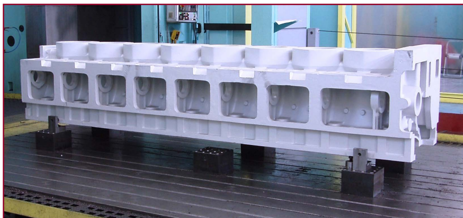
SinterCast's largest casting during 2013 was a 9 tonne engine entablature for Allen Diesels of the UK. With CGI entablatures and heads, the Allen Series 4000 engines provide power outputs from 1,800 to 5,050 kWe in power generation applications around the world. (Courtesy Allen Diesels)
