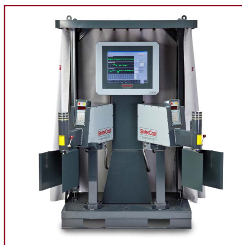
System 3000 with two Sampling Modules
