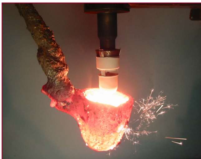
SinterCast's unique immersion sampling
