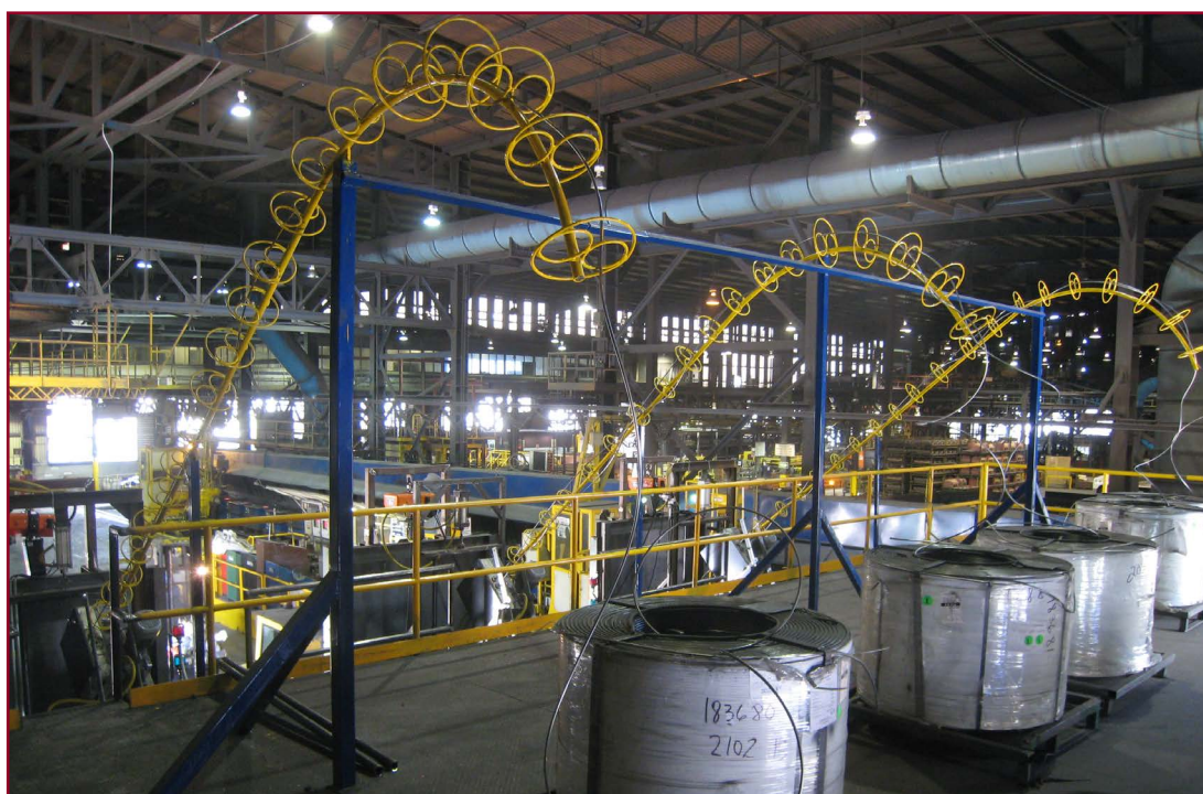
System 3000 Plus: multiple wirefeeders for base treatment and correction at the Tupy Saltillo foundry in Mexico (Courtesy, Tupy)
