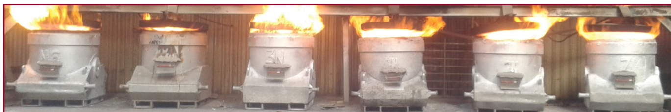
Figure 6: RFID tags or 2D optical matrix plates enable ladles to be traced throughout the process, linking each mould to the liquid metal history
