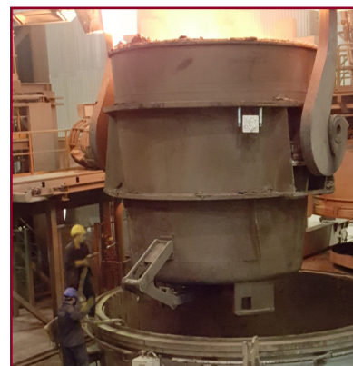
Figure 3: RFID tags or 2D optical matrix plates (shown) can be used to identify ladles
