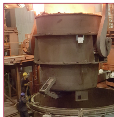
RFID tags or 2D optical matrix plates (shown) can be used to identify ladles.
