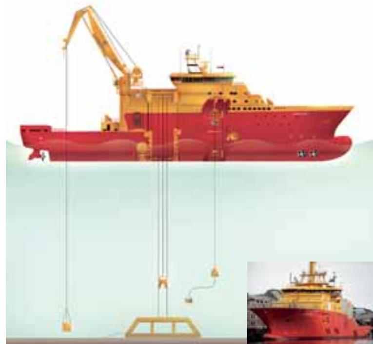
**Research and development** The challenging nature of offshore operations means that load handling must often be undertaken by a wide variety of specialised systems, not just cranes. Many subsea lifts require advanced module handling systems which can offer very precise handling of critical loads – something which is vital when mating subsea units on the seabed or in the vicinity of other delicate equipment. This precision becomes even more challenging in rough seas.
