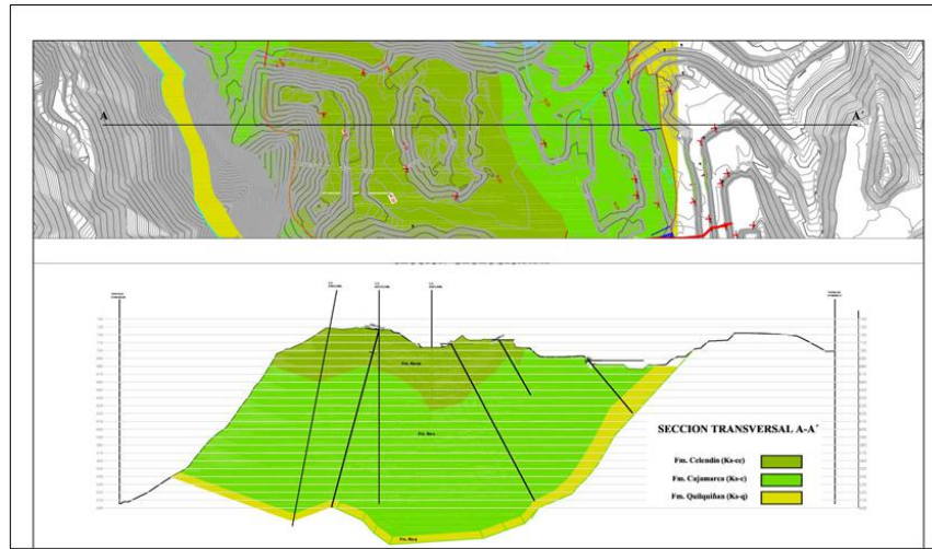
Figure 6 Geological Section of the Tembladera quarry
