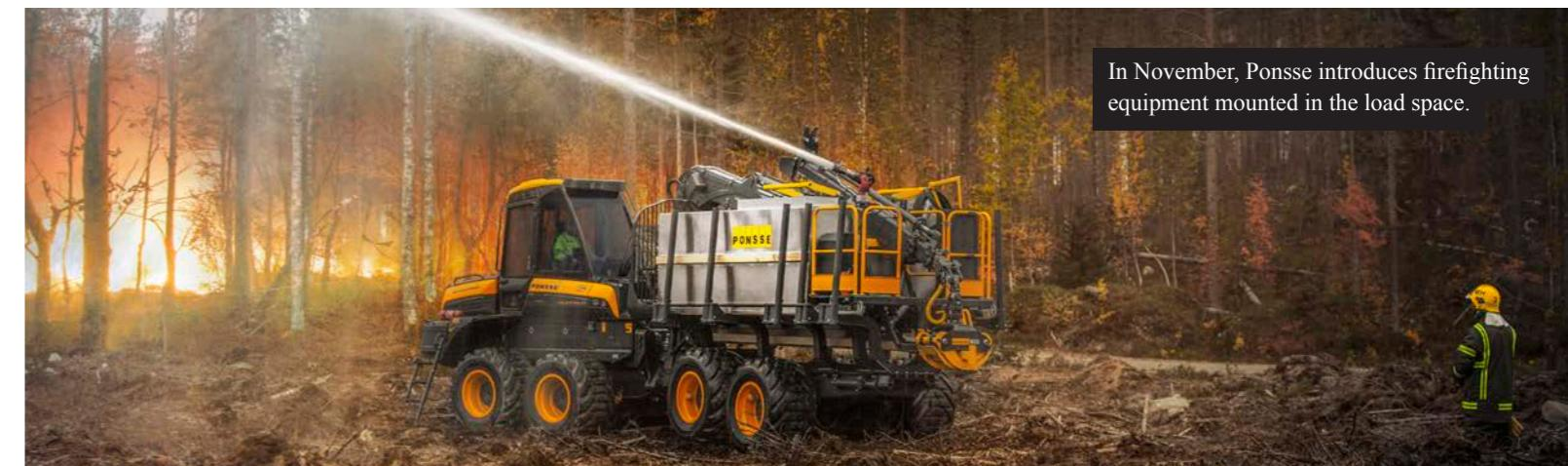
In November, Ponsse introduces firefighting equipment mounted in the load space.
